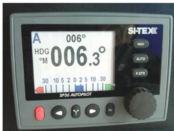
The SP36 is the first SI-TEX autopilot to offer full Virtual Feedback capabilities, eliminating the need for a rudder feedback unit when installed on outboard powered or stern drive vessels. SI-TEX's Virtual Feedback feature makes installation of the SP36 straightforward and uncomplicated and improves reliability of the overall system by eliminating a critical part. For commercial vessels that use a rudder feedback unit, the SP36 is available with full "fly by wire" follow-up steering levers.
